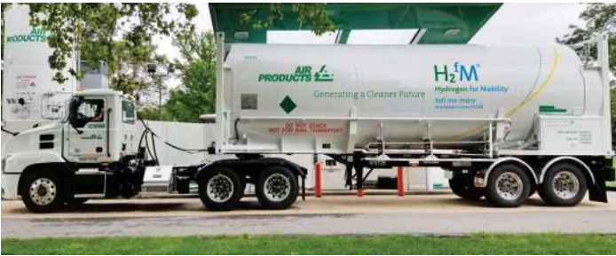
Figure 2. Air Products liquid hydrogen tanker for hydrogen bulk deliveries.
