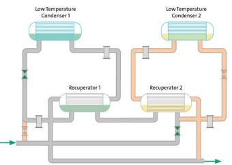
Figure 2: Schematic of a Cryo-Condap<sup>®</sup> installation at a biopharmaceutical manufacturing site with recuperators used to pre-cool the incoming waste gas stream.
