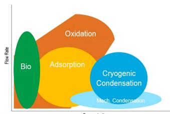
Concentration Figure 1: Alternative types of technology for solvent abatement and VOC recovery
